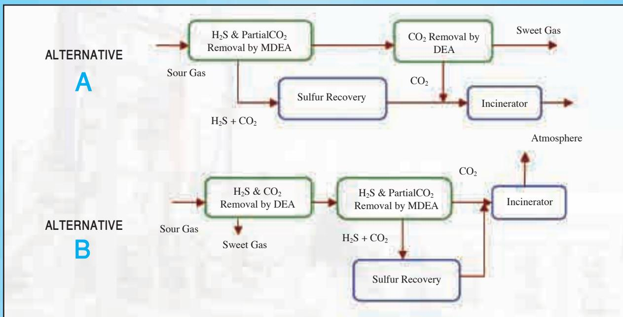
Figure 1: Schematic diagram for alternatives of acid gas removal
